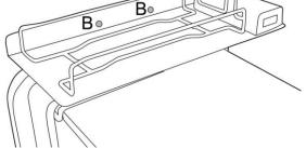
2. Once the main body is in place, hold the head section flush to the top of the ironing board and mark the positions (B) on the wall. Drill holes at the marked positions suitable for the fixings used. Re-align the head section and fix in place using an electric screw driver (recommended).
