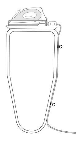
3. Fix the mains lead along the side of the back board at points (C) using the clips provided.
